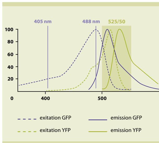
Figure 2: The excitation and emission spectra of GFP (blue) and YFP (green). Shaded area represents the bandpass filter used for collection of the emission spectra of GFP and YFP. The V2 and B1 channels of the MACSQuant VYB both use the 525/50 filter which enables detection of GFP and YFP separately.
